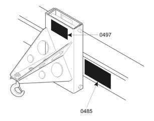
Figure 8-7. Material Lifting Hook Decals
